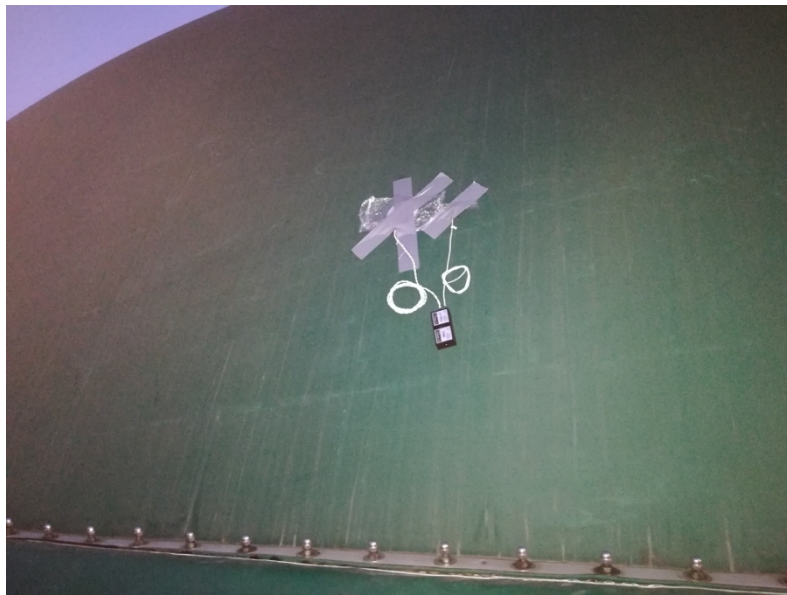
Fig. 4 The device used for the determination of heat fluxes placed on the surface of the HSs gasometric coverage system.
